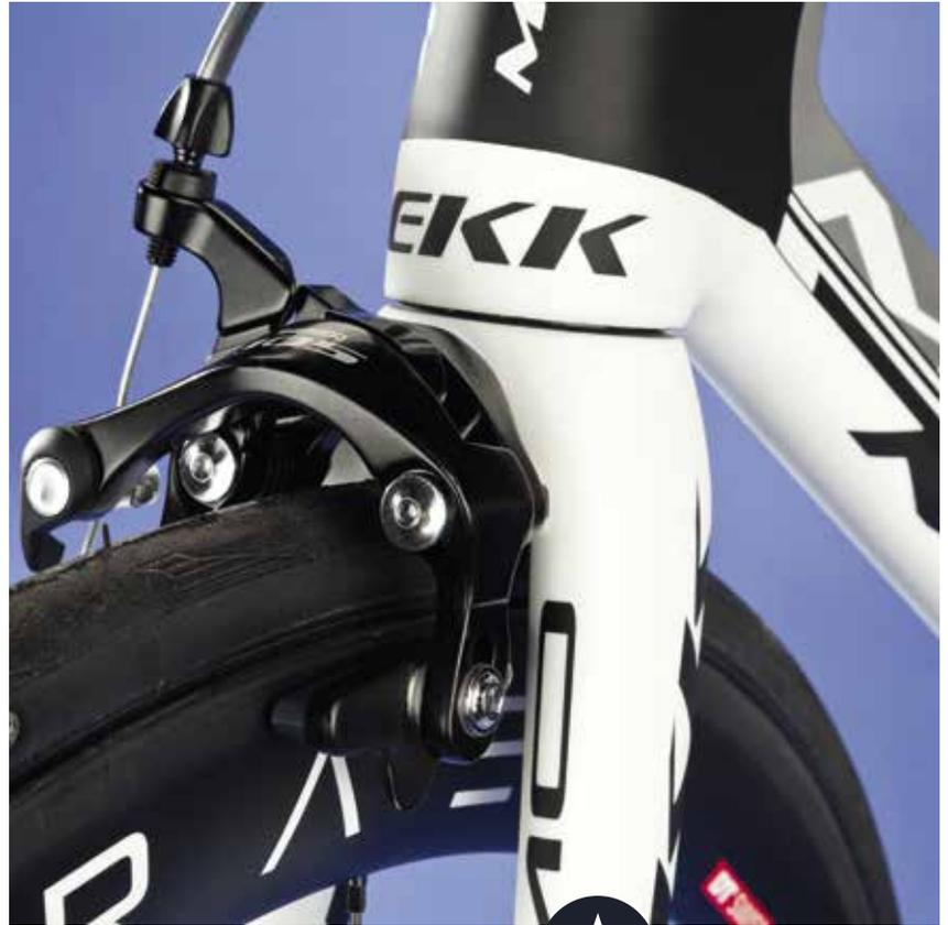
they're not perfectly suited to the full carbon braking surface of the bike's deep-section wheels.
