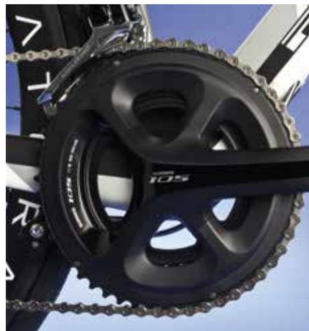
The Primo 6.2 employs a full 105 groupset (above); seatstays join the seatpost well below the top tube (right), while a cutout allows a very short wheelbase
